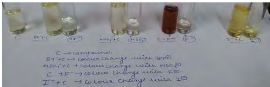
Figure 6. Detection of fluoride ion by thiourea based receptor 2.
