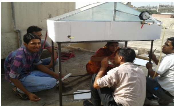
Preliminary work being carried out by students to fabricate solar water distiller
