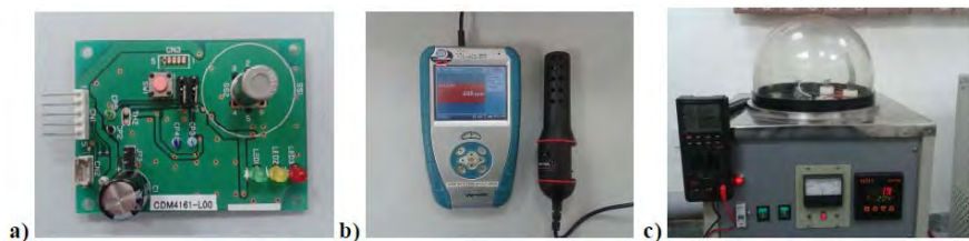
a) Figaro CO 2 sensor b) Vernier CO 2 sensor with data acquisition module c) Gas Sensing Test Rig (GSTR) for simulation of controlled environmental conditions
